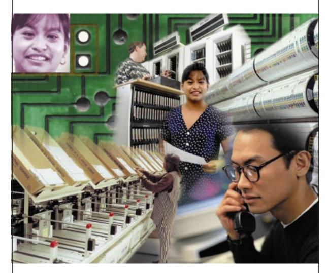
(Center) The Automatic Cartridge Loader is a component of a laser printing system which provides faster and more cost efficient printing of taxpayer communications. (Upper Right) Computer tape reels are used for storing the output from taxpayer return processing. This form of media storage is being replaced by cartridge tapes and automated tape libraries as part of the IRS modernization strategy.
